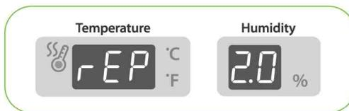
▶ Press **(O.K)** button to remove buzzer and alarm indication. (Buzzer will be removed automatically after 15sec.)
