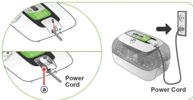
▶ In case of connecting power cord of incubator, incubation starts at the existing set temperature and humidity. [temperature of initial shipment 26.1°C (78.98°F)]
