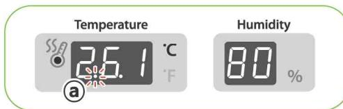
**Tip** Quick Start : If you just connect power, it automatically starts incubation with factory setting. [Factory setting : Temperature 26.1°C (78.98°F)]
