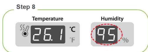
EX : ↔ ※ It displays that its inside humidity was temporarily higher than abnormal high humidity alarm set value(RH 95%) during incubation.
